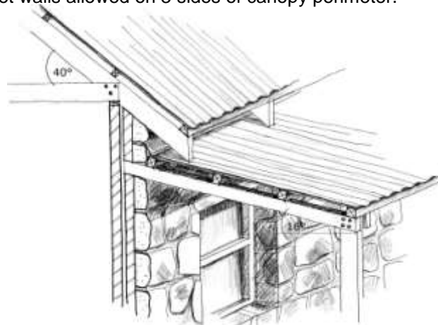
Detail of roof overhang with canopy
